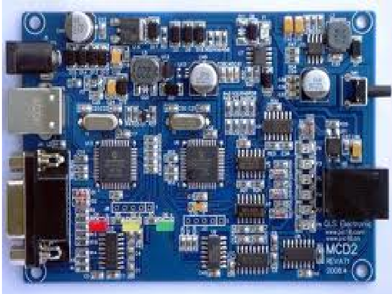
Figure 2. Example of SMT assembly
